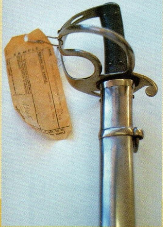
Fig 1. Sealed Pattern 1853 sword; SP 236. The back of the 35 and 1/2 ins. blade is stamped "ENFIELD" and the outer face of the scabbard is stamped with "crown" over "E" over "6" and "ENFIELD". This was the first universal troopers sword for all Line Cavalry. (Ministry of Defence Pattern Room, Nottingham).
